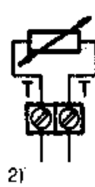
Fig. 4. Collegamento di sonde termiche bimetalliche, sonde termiche a termistori (PTC), scaldiglia anticondensa Connection of bi-metal type thermal probes, thermistor type thermal probes (PTC), anti-condensation heater
